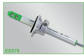
The alignment strip along the probe's tube and the matching mounting flange determine the orientation of the sensor probe. The mounting flange allows for an infinitely variation of the depth of the sensor probe. The electronics integrated in the probe tube provide a linear analogue signal of 0-5V or 0-10V for the velocity range 0...1m/s (0...200ft/min) or 0...2m/s (0...400ft/min).
